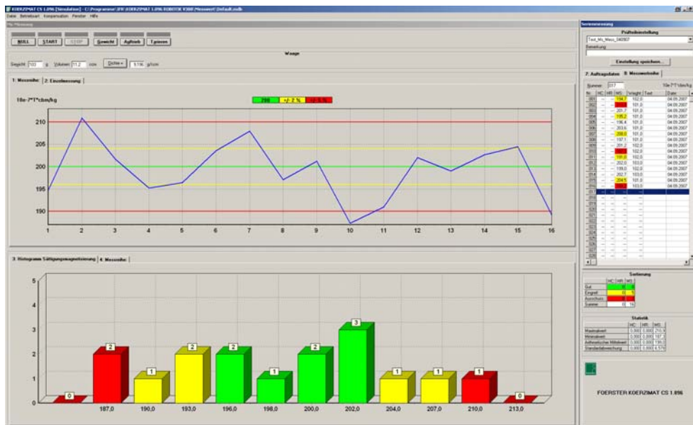
Fig. 8 User interface: serial measurement Ms with displayed line graph, histogram and table of the measured values
